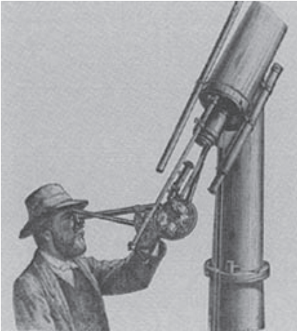
Figure 33: Norman Lockyer using a spectroscope attached to a telescope.
