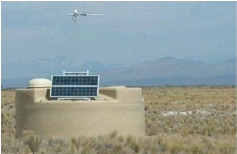
Figure 79: A water tank detector in the Pierre Auger cosmic ray observatory.
