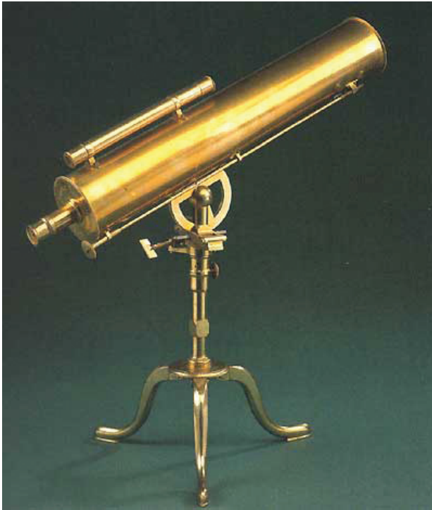
Figure 23: A reflecting telescope built by James Short, using the Gregorian design. A 'finder' telescope, mounted on top of the main tube, was used to point the tube in the right direction.
