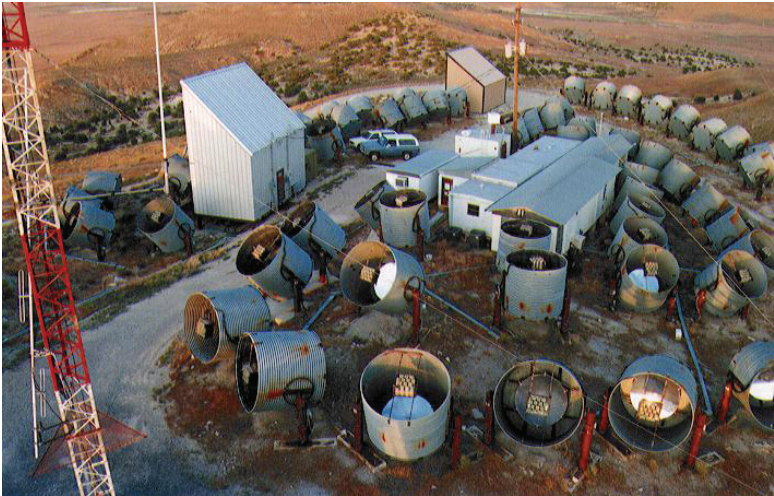
Figure 78: The Fly's Eye observatory in Utah, USA, observes Cerenkov radiation from cosmic rays crossing different parts of the sky.
