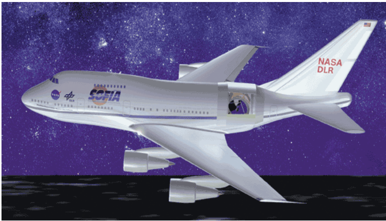
Figure 69: SOFIA carried an infrared telescope to the stratosphere.
